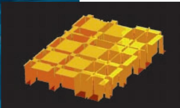
*Diffractive fan-out structures are used for multiple beam generation.*
