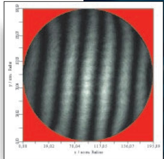
*The ability to measure micro-optics is crucial to achieve a quality product. The interferogram shows a microlens with diffraction limited quality.*
