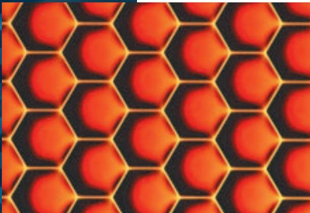
*Hexagonal lens arrays provide very high fill factors with minimal space between the lenses.*
