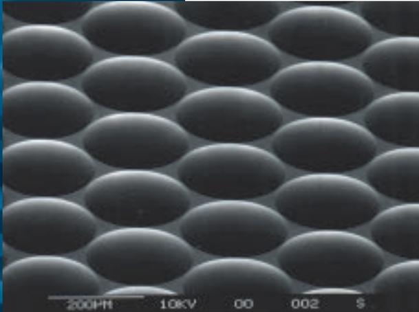
*Refractive lens arrays are provided in a range of diameters and focal lengths.*
