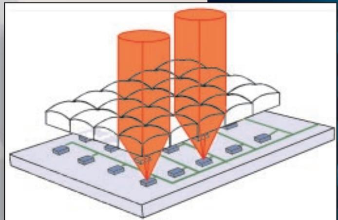
*An important application of microlens arrays is fill factor enhancement in CCD cameras.*
